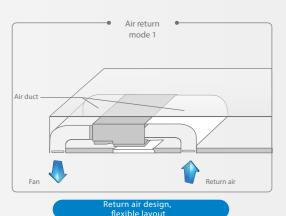
Multiple air return types can be achieved through simple adjustment, providing a greater degree of freedom in the installation process.
